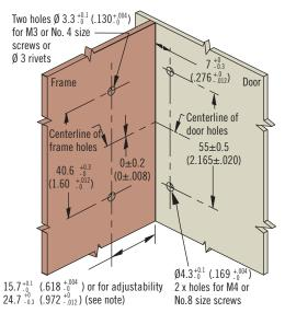
Note: These holes and dimensions are used only if adjustability through the use of slotted holes in catch is desired.
