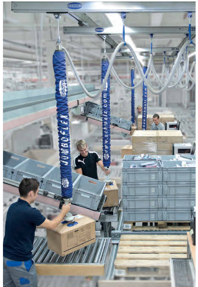
Aluminum multi bridge crane system with vacuum tube lifters JumboFlex commissioning packages
