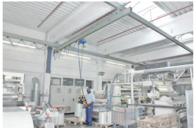
Aluminum multi bridge crane system with reinforced section and chain hoist handling rolls of film
