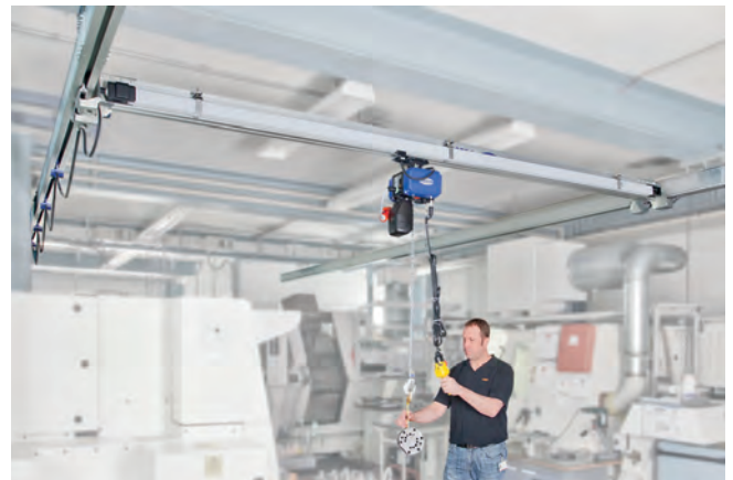
Low ceiling mounted aluminum single bridge crane system with conductor line to accommodate the low ceiling height
