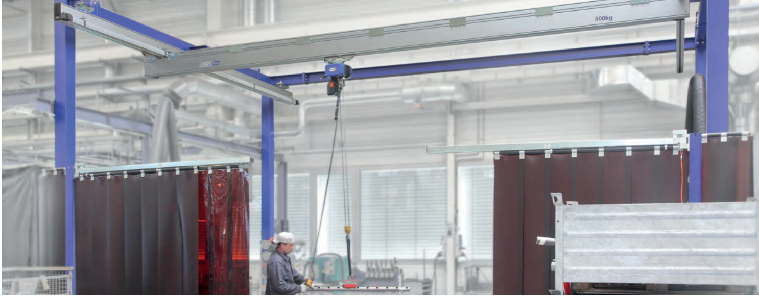
Aluminum single bridge crane system with reinforced section and a conductor line used with a chain hoist and a magnet
