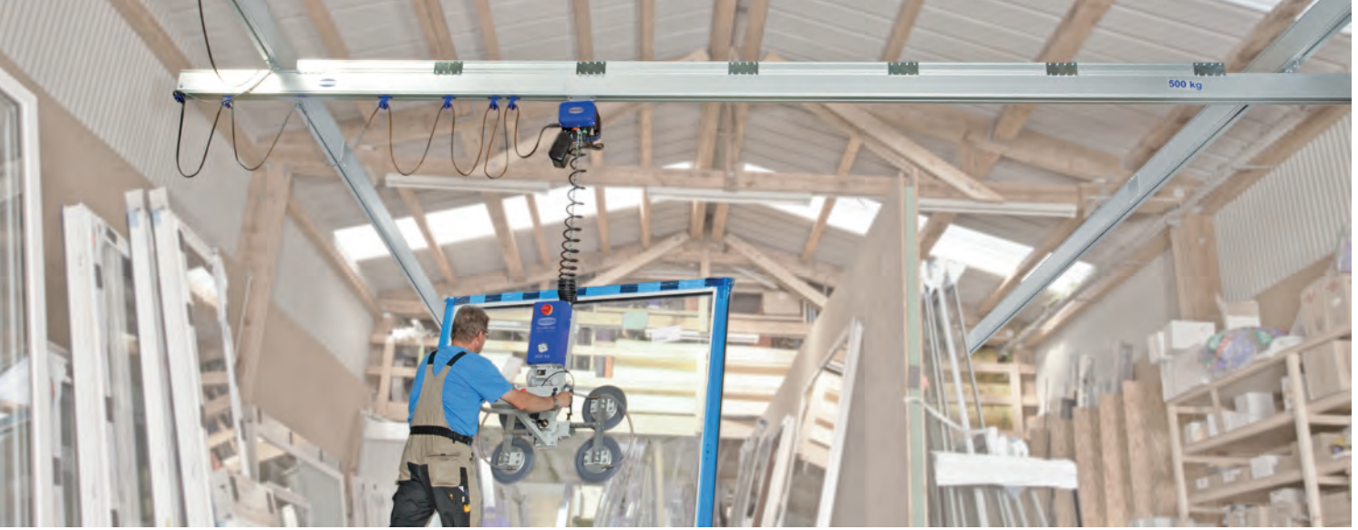
Aluminum single bridge crane system with reinforced section and vacuum lifting device VacuMaster Window during handling of windows
