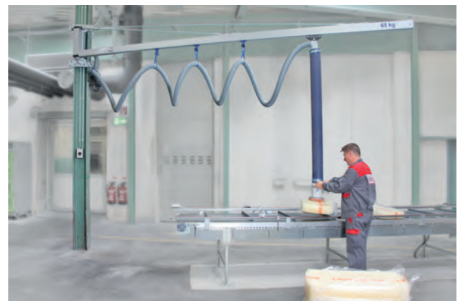
Aluminum wall mounted jib crane, mounted to a production hall pillar, with vacuum tube lifter JumboSprint during handling of raw rubber bales
