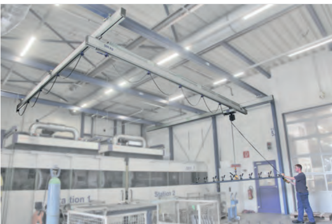
Aluminum single bridge crane system with reinforced section and chain hoist during machine loading
