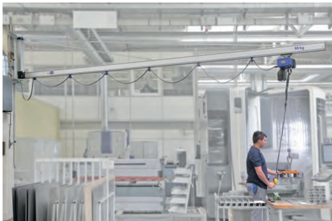
Aluminum wall mounted jib crane with chain hoist and magnet during loading of a milling machine
