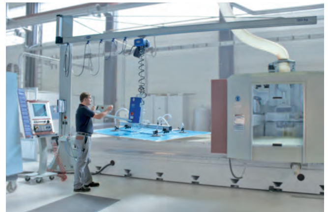
Aluminum column mounted jib crane with vacuum lifting device VacuMaster Comfort during loading of a CNC machining center
