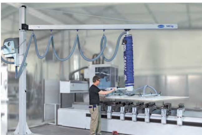
Aluminum column mounted jib crane with vacuum tube lifter JumboErgo during loading of a CNC machining center
