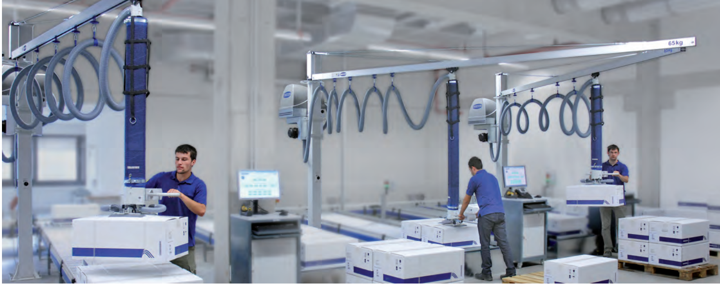
Aluminum column mounted jib cranes with vacuum tube lifters JumboErgo during the commissioning of packages
