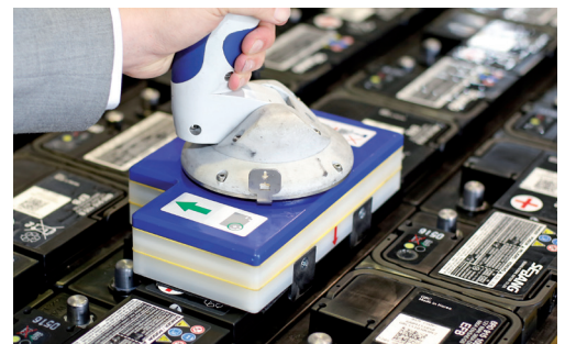
Whether closely stacked or types of batteries. Both can easily be handled with only one Vacuum-Gripper from above
