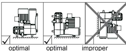
Clearance between compressors and adjacent walls should be no less than 10 cm of free space in order to ensure sufficient air flow for cooling. Schmalz GmbH prior to installation under noise insulation canopies, contact.
