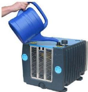
**Pour an additional 1.5l operating liquid into the suction nozzle (pos. A) of the system, so that operating liquid enters the interior of the integrated unit.**
