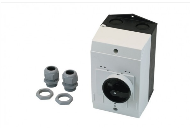
MSS-K 1.6-2.5A Part no. 10.04.04.00119 Motor-protection switch with housing Current range: 1.6 ... 2.5 A Actuation: Rotary switch Colour: grey Protection: IP 65
