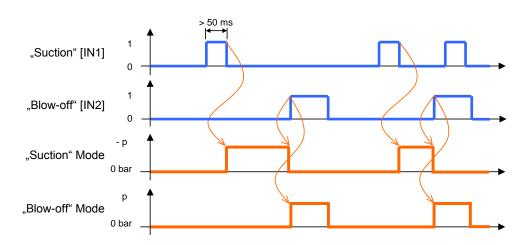
IMP ejectors are set to "pneumatically OFF" on delivery. The ejector only begins suction after a valid pulse is received via the suction signal input.
