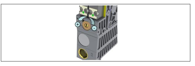
A valve screw is located underneath the pilot valve. This valve screw can be used to set the blow-off volume flow.
