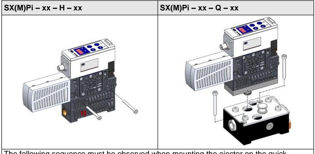
The following sequence must be observed when mounting the ejector on the quickchange system:
