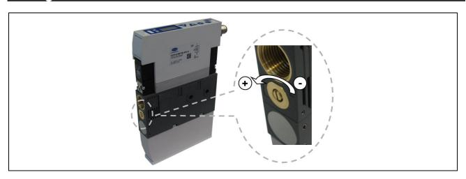
The valve screw for setting the blow-off volume flow is located underneath the vacuum connection. The volume flow is reduced by turning the valve screw clockwise and increased by turning it anti-clockwise. The valve screw is equipped with a stop on both sides.
