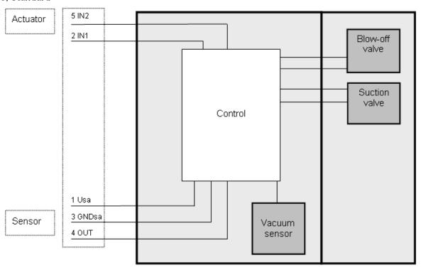
Terms refer to the pin layout of the M12-5 or the M12-8 S connector
