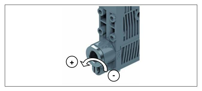
There is a valve screw below the vacuum connection (2). This valve screw can be used to set the blow-off volume flow.
