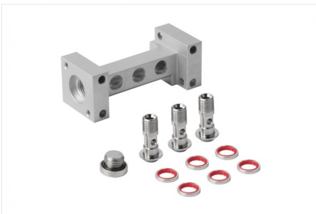
GP 3 SCPS 07..15 G2 Part no. 10.02.02.04884 Compressed-air distributor for use as a manifold and for building ejector blocks Number of connections: 3 Length L: 89.4 mm Width B: 38 mm Height H: 34 mm for: Ejector SCPS 07..15 G2
