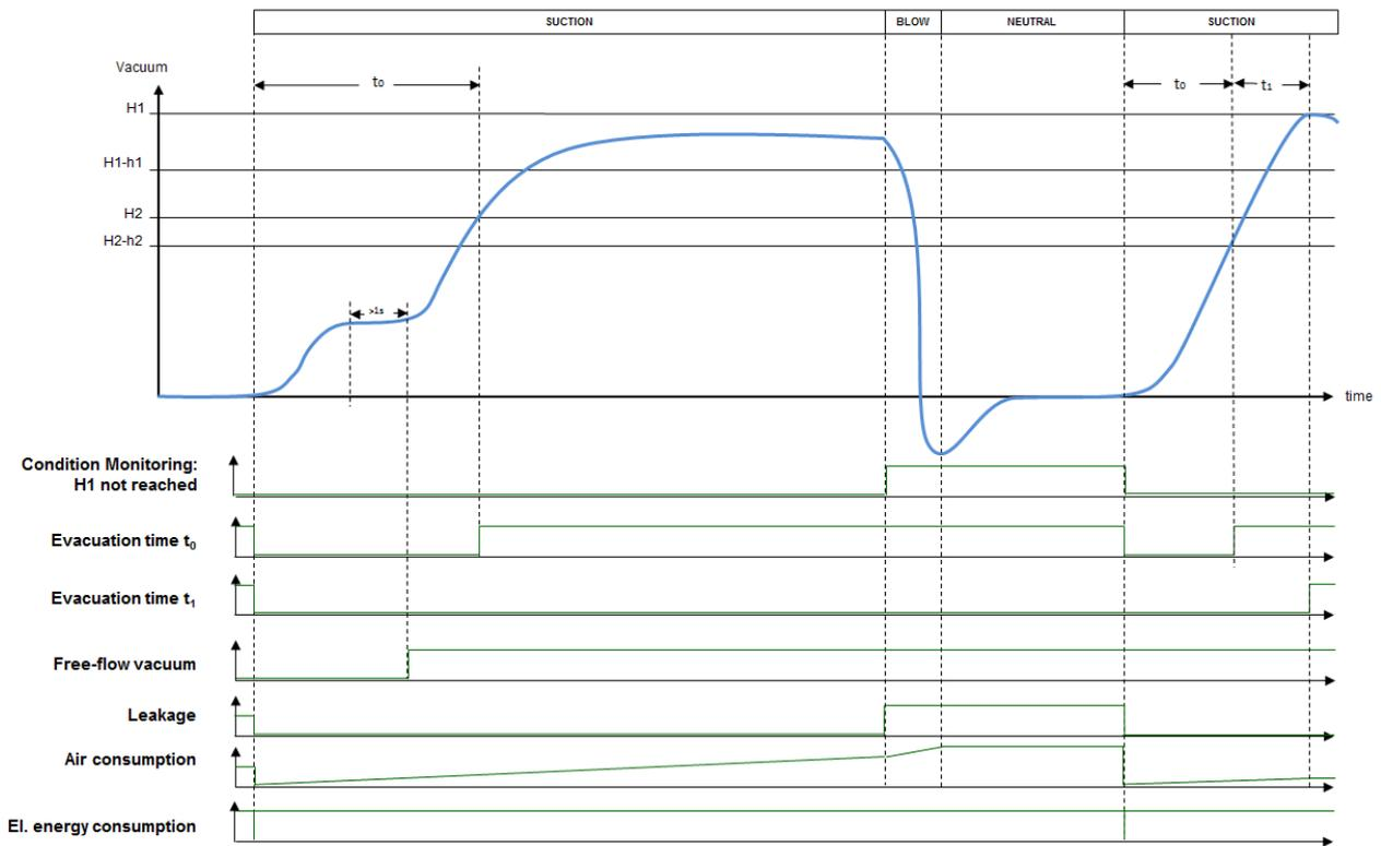
Handling cycle with excessive evacuation time  $t_1$
