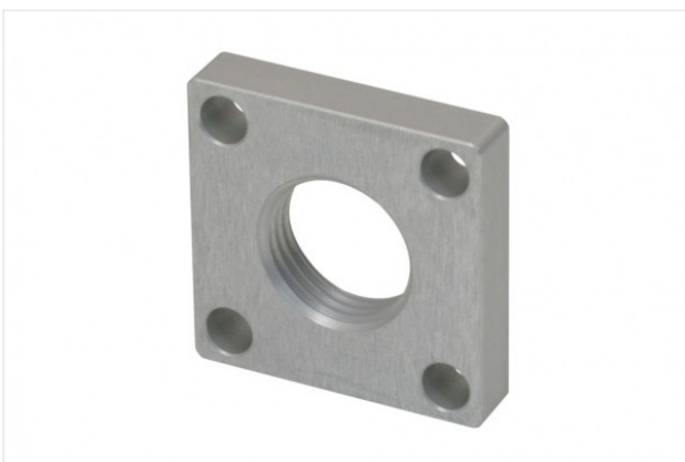
VRS-PL-40 G1/2-IG MO-PROF Part no. 25.09.06.00009 Sealing plate Length: 40 mm Height: 10 mm Thread 1: G1/2-F for: Mounting section
