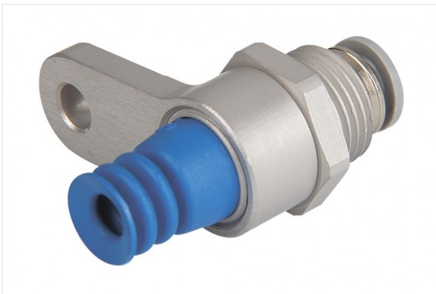
SD-MOD 4 32x15x35 FG 9 SWGm Part no. 10.01.30.00121 Suction-/ Absorption module Internal diameter: 4 mm Length: 32 mm Width: 15 mm Height: 35 mm Hose diameter: 4 mm Suct. pads: Bellows suct. pad FG Diameter: 9 mm for: Wafer gripper (mod)
