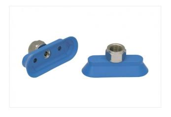
Dimensions (LxB): 80 x 30 mm Suction cup material: Nitrile rubber NBR Material hardness: 45 °Sh Nipple material: Brass, nickel-plated Vacuum connection: G3/8-F
