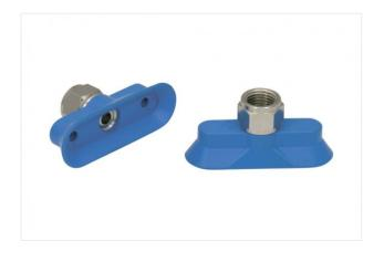
Dimensions (LxB): 60 x 20 mm Suction cup material: Nitrile rubber NBR Material hardness: 45 °Sh Nipple material: Brass, nickel-plated Vacuum connection: G1/4-F
