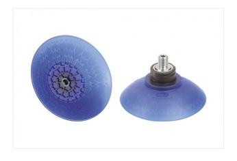
Size: 115 Suction cup material: Elastodur Material hardness: 85 °Sh Vacuum connection: G1/4"-M Nipple material: Aluminium
