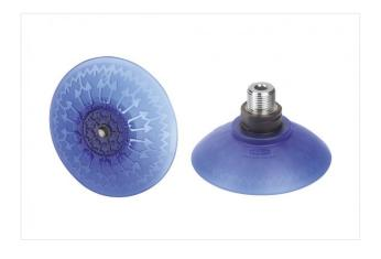
Size: 80 Suction cup material: Elastodur Material hardness: 85 °Sh Vacuum connection: G3/8"-M Nipple material: Aluminium
