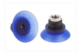
Size: 50 Suction cup material: Elastodur Material hardness: 85 °Sh Vacuum connection: G1/4"-F Nipple material: Brass, nickel-plated
