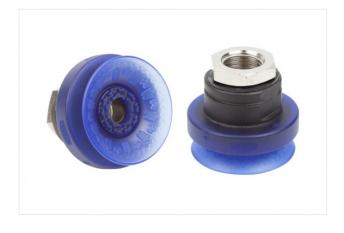
Size: 40 Suction cup material: Elastodur Material hardness: 85 °Sh Vacuum connection: G1/4"-F Nipple material: Brass, nickel-plated
