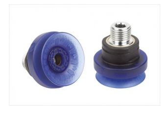
Size: 30 Suction cup material: Elastodur Material hardness: 85 °Sh Vacuum connection: G1/4"-M Nipple material: Aluminium
