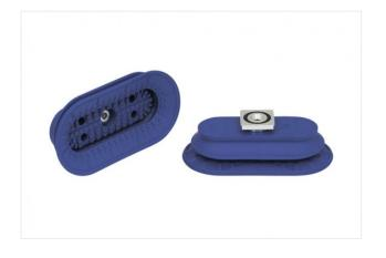
Dimensions (LxB): 140 x 70 mm Suction cup material: Nitrile rubber NBR Material hardness: 60 °Sh Nipple material: Aluminium Vacuum connection: Rectangular adapter Number of folds: 1.5
