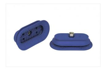
Dimensions (LxB): 140 x 70 mm Suction cup material: Nitrile rubber NBR Material hardness: 60 °Sh Nipple material: Brass, nickel-plated Vacuum connection: G1/4-F Number of folds: 1.5
