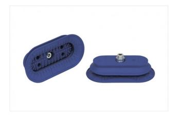
Dimensions (LxB): 140 x 70 mm Suction cup material: Nitrile rubber NBR Material hardness: 60 °Sh Nipple material: Aluminium Vacuum connection: G1/4-M Number of folds: 1.5
