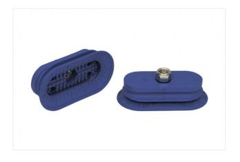
Dimensions (LxB): 110 x 55 mm Suction cup material: Nitrile rubber NBR Material hardness: 60 °Sh Nipple material: Brass, nickel-plated Vacuum connection: G1/4-F Number of folds: 1.5
