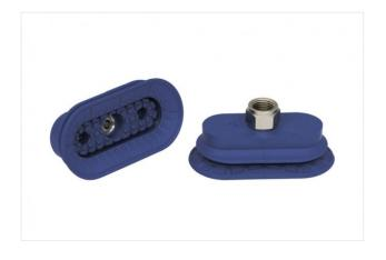
Dimensions (LxB): 80 x 40 mm Suction cup material: Nitrile rubber NBR Material hardness: 60 °Sh Nipple material: Brass, nickel-plated Vacuum connection: G1/4-F Number of folds: 1.5
