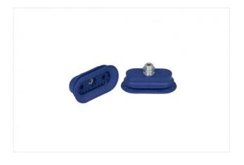
Dimensions (LxB): 80 x 40 mm Suction cup material: Nitrile rubber NBR Material hardness: 60 °Sh Nipple material: Aluminium Vacuum connection: G1/4-M Number of folds: 1.5
