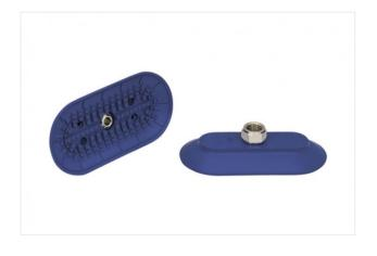
Dimensions (LxB): 140 x 70 mm Suction cup material: Nitrile rubber NBR Material hardness: 60 °Sh Nipple material: Brass, nickel-plated Vacuum connection: G3/8-F
