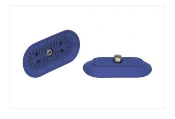
Dimensions (LxB): 140 x 70 mm Suction cup material: Nitrile rubber NBR Material hardness: 60 °Sh Nipple material: Brass, nickel-plated Vacuum connection: G1/4-F
