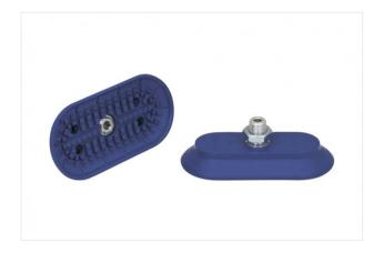
Dimensions (LxB): 120 x 60 mm Suction cup material: Nitrile rubber NBR Material hardness: 60 °Sh Nipple material: Aluminium Vacuum connection: M14x1.5-M
