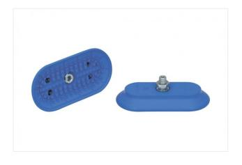
Dimensions (LxB): 120 x 60 mm Suction cup material: Nitrile rubber NBR Material hardness: 45 °Sh Nipple material: Steel Vacuum connection: M10-M
