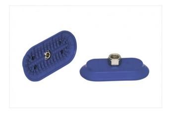
Dimensions (LxB): 120 x 60 mm Suction cup material: Nitrile rubber NBR Material hardness: 60 °Sh Nipple material: Brass, nickel-plated Vacuum connection: G3/8-F
