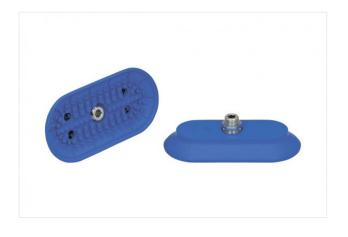
Dimensions (LxB): 120 x 60 mm Suction cup material: Nitrile rubber NBR Material hardness: 45 °Sh Nipple material: Aluminium Vacuum connection: G1/4-M
