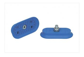
Dimensions (LxB): 100 x 50 mm Suction cup material: Nitrile rubber NBR Material hardness: 45 °Sh Nipple material: Steel Vacuum connection: M10-M
