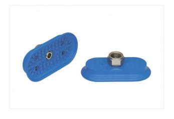
Dimensions (LxB): 100 x 50 mm Suction cup material: Nitrile rubber NBR Material hardness: 45 °Sh Nipple material: Brass, nickel-plated Vacuum connection: G3/8-F
