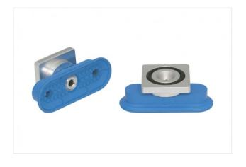
Dimensions (LxB): 60 x 23 mm Suction cup material: Nitrile rubber NBR Material hardness: 45 °Sh Nipple material: Aluminium Vacuum connection: Rectangular adapter
