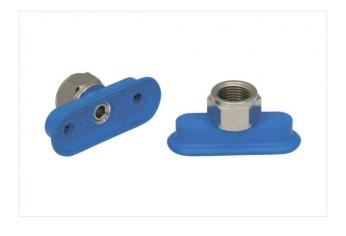
Dimensions (LxB): 60 x 23 mm Suction cup material: Nitrile rubber NBR Material hardness: 45 °Sh Nipple material: Brass, nickel-plated Vacuum connection: G3/8-F
