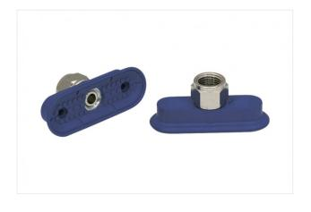
Dimensions (LxB): 60 x 23 mm Suction cup material: Nitrile rubber NBR Material hardness: 60 °Sh Nipple material: Brass, nickel-plated Vacuum connection: G1/4-F
