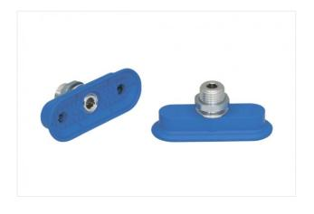
Dimensions (LxB): 60 x 23 mm Suction cup material: Nitrile rubber NBR Material hardness: 45 °Sh Nipple material: Aluminium Vacuum connection: G1/4-M
