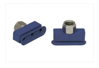
Dimensions (LxB): 50 x 16 mm Suction cup material: Nitrile rubber NBR Material hardness: 60 °Sh Nipple material: Brass, nickel-plated Vacuum connection: G1/4-F
