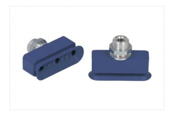
Dimensions (LxB): 50 x 16 mm Suction cup material: Nitrile rubber NBR Material hardness: 60 °Sh Nipple material: Aluminium Vacuum connection: G1/4-M
