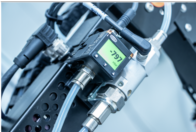
Vacuum and pressure switch VS-V/VP-W for measuring and monitoring on suction spider
