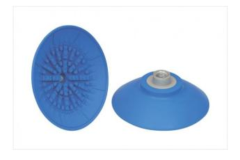
Size: 125 Suction cup material: Nitrile rubber NBR Material hardness: 45 °Sh Vacuum connection: G3/8-F Nipple material: Aluminium
