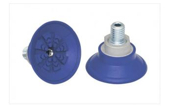
Size: 40 Suction cup material: Nitrile rubber NBR Material hardness: 60 °Sh Vacuum connection: M10-M Nipple material: Steel
