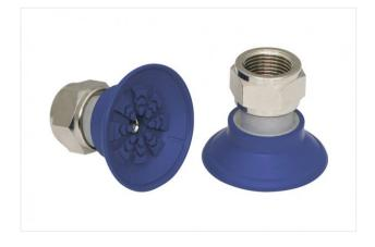
Size: 40 Suction cup material: Nitrile rubber NBR Material hardness: 60 °Sh Vacuum connection: G3/8-F Nipple material: Brass, nickel-plated
