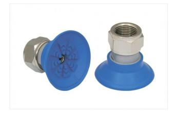
Size: 40 Suction cup material: Nitrile rubber NBR Material hardness: 45 °Sh Vacuum connection: G3/8-F Nipple material: Brass, nickel-plated
