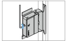
Closing speed is adjustable with a hex key. (size: 2.5)
