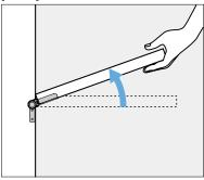
The lock will be released if the angle is more than  $90^{\circ}$  .
