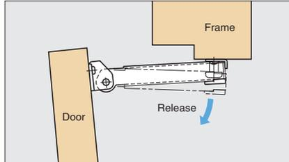
• Release the door guard as above to close the door completely.
