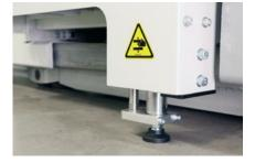
The support feet extend automatically after the jib is unlocked, minimizing cycle times.
