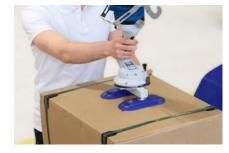
The tube lifter is started at the push of a button. It can be combined with various quick-change grippers.
