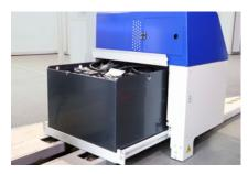
The large capacity battery can be charged in the device and is also easy to change for multi-shift operation.
