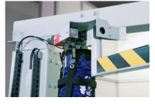
A magnetic switch fixes the jib in a safe parking position during transport.
