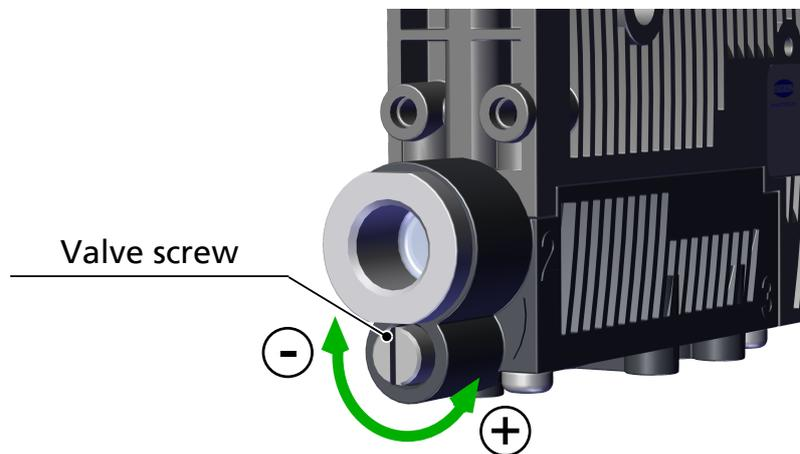
1. Turn the valve screw clockwise to reduce the flow rate.
